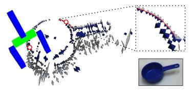
Fig. 2: Grasp reflex based on visual data. Each ECV descriptor is rendered with a small plane patch. Patch normals are not part of ECV descriptors; they are arbitrarily defined for the purpose of 3D rendering.
